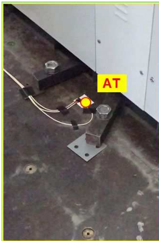
Photo 4: AT Reference point placed on the shaking table
