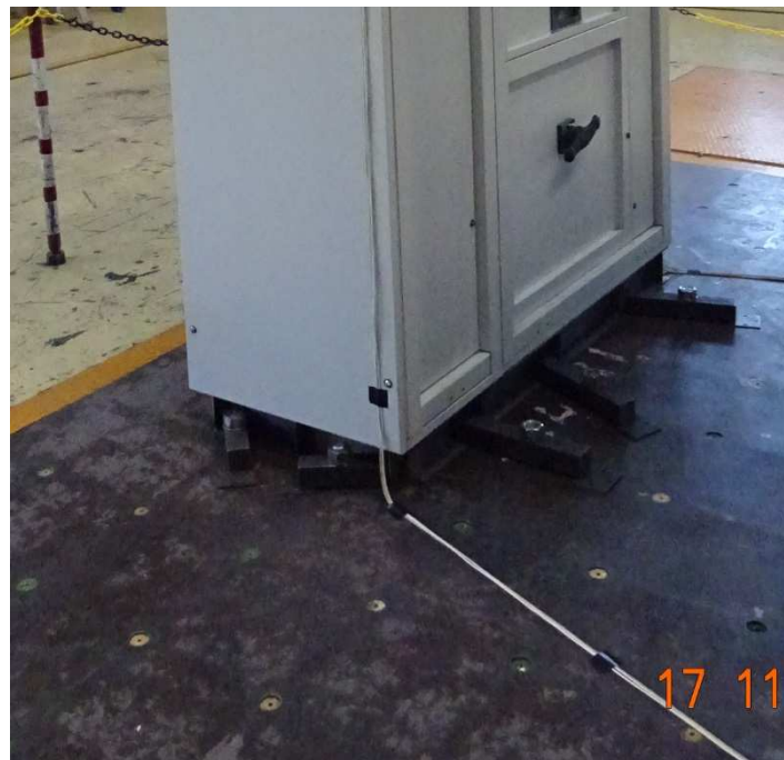
Photo 2: Fixing of Unit to shaking table
