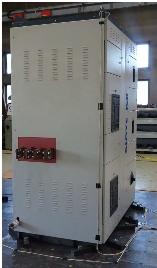
Photo 2: Fixing of Unit to shaking table
