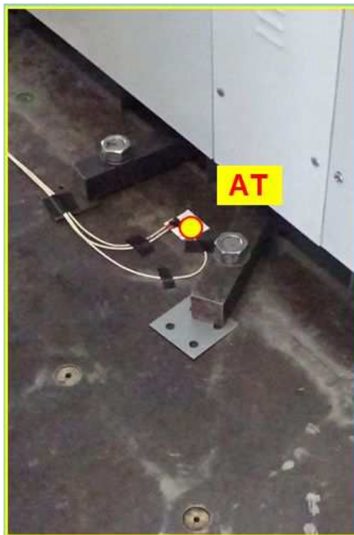
Photo 5: A3 Measuring point placed on the switchgear support
